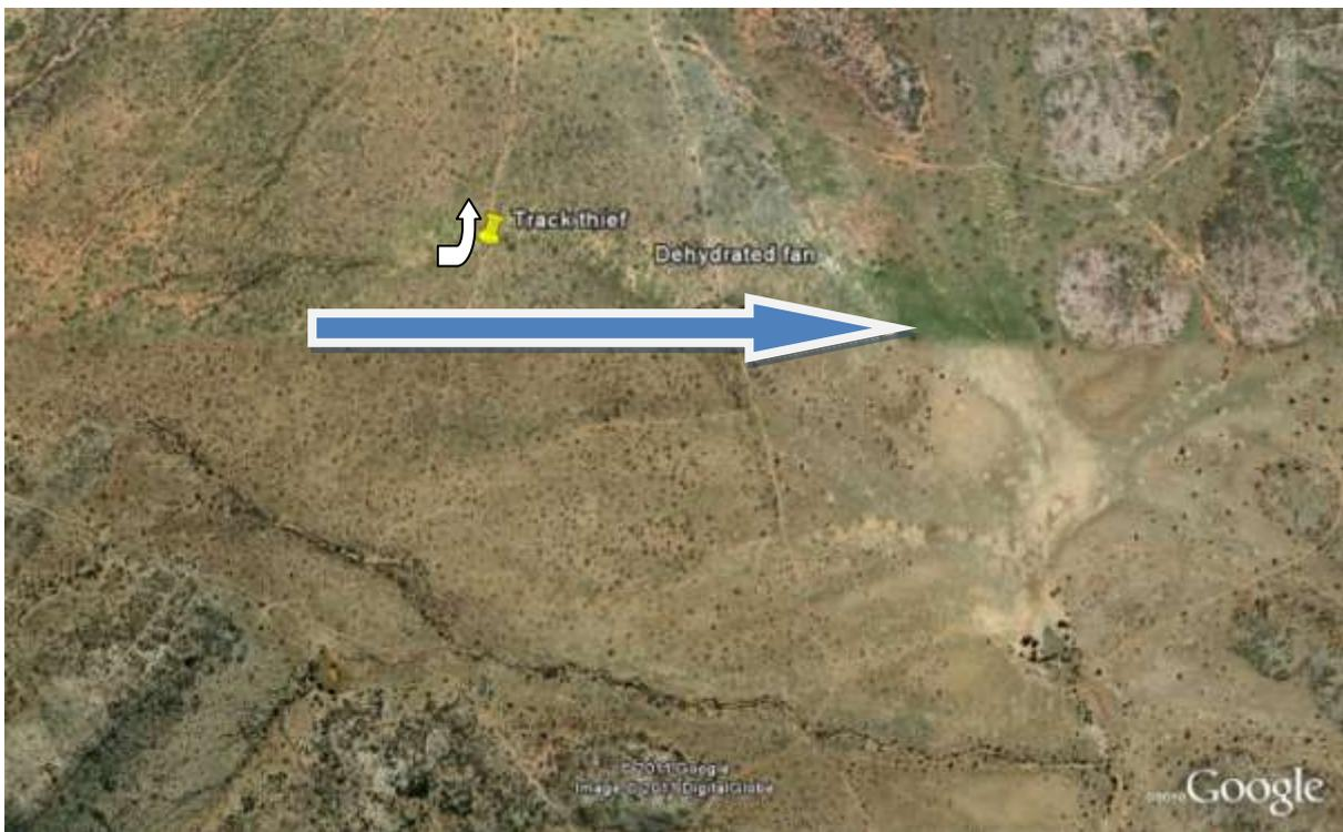
**Figure 1. A farm road is intercepting flow (“Track thief”) and sending it to the north, into a different catchment. This leaves the area below starved of sheet flow (“Dehydrated fan”)**
