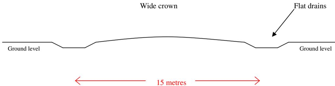
Wide formed roads are easier, quicker and cheaper to maintain. Water flows are less confined and there is less soil loss.
