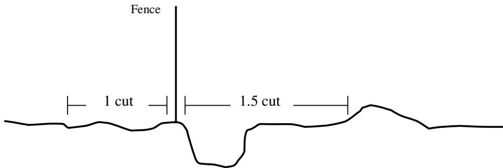
➤ Cross-section before treatment. As erosion occurs, operators widen grading.
