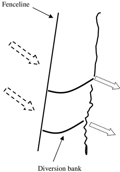
➤ Single track with speed bump (diversion bank) installed.
