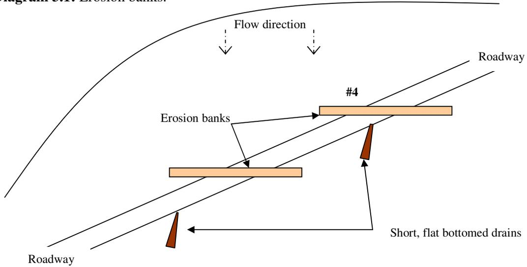
Erosion banks can be installed over a formed road, but care must be taken to ensure area #4 is level/flat so that no water is contained.
