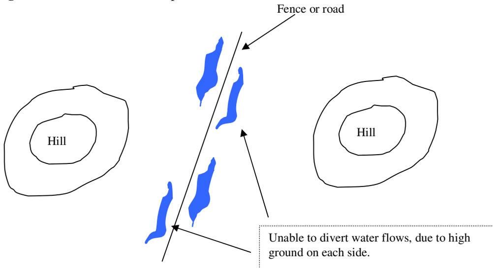
Solution: Often the only method is to relocate the infrastructure and follow the contour line closer, enabling water flow to "cross" the line.
