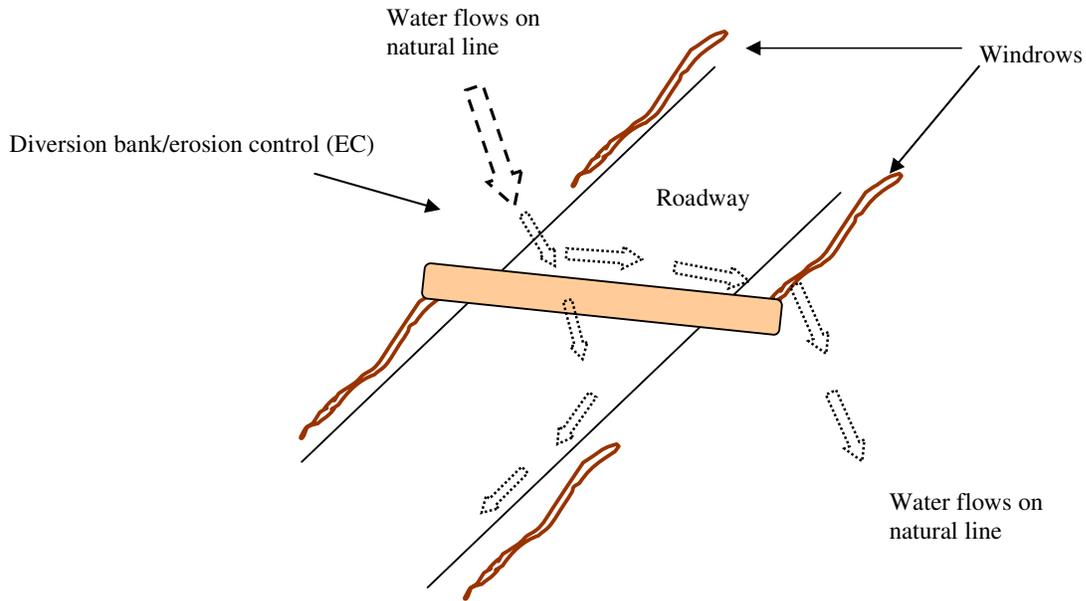
A grader/loader can often scrape/push these unused soils into small banks across the roadway, thereby enabling water flows to get back to their original direction. This method clears away the windrows and provides necessary soils without having to cut into further ground levels.
