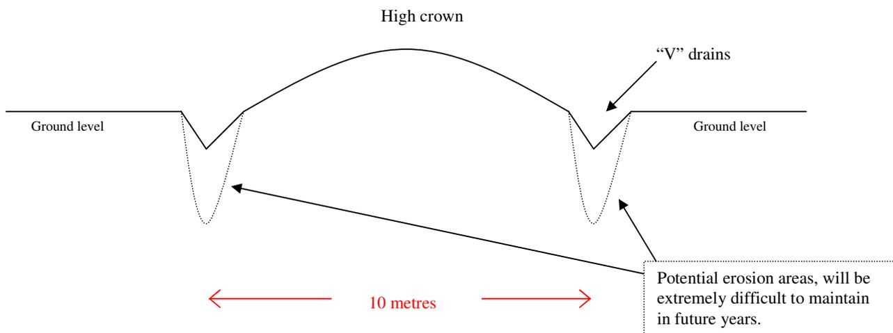
A high crown can be very unstable for traffic when slippery and traffic is usually confined to set "tracks" which assist in erosion of the roadway crown.
