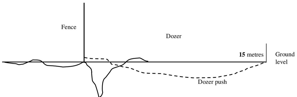
➤ Dozers tend to work over a short distance resulting in a deep depression parallel to the fence.
