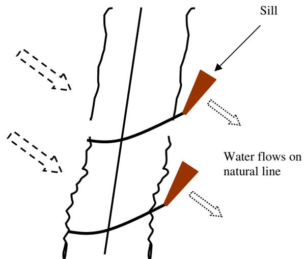
The greatest cause of fenceline and access track erosion is that the windrows channelling waterflows in directions away from the natural drainage line.
